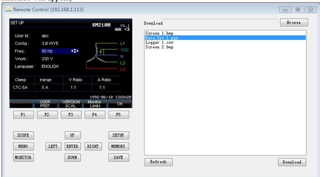
Remote control the device through pressing buttons in left area of above interface, the right area is the stored list files, user can click 'Download' button to download selected files to the computer.
