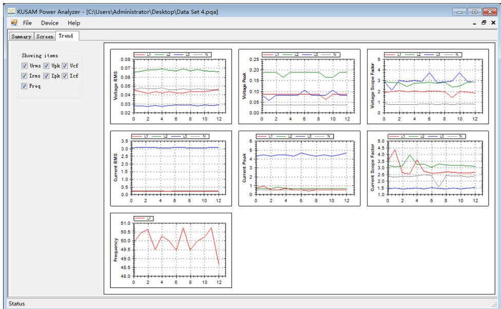
(3) Open log file with .csv format, user can directly open EXCEL file under windows or open it using this software. Click Y zoom button and then click data table, scroll up or down the mouse wheel to realize the zooming of Y-axis only. Click X zoom button and then data table, scroll up or down the mouse wheel to realize the zooming of X-axis only. Hold the mouse left clicking to make the left or right shifting of data waveform.
