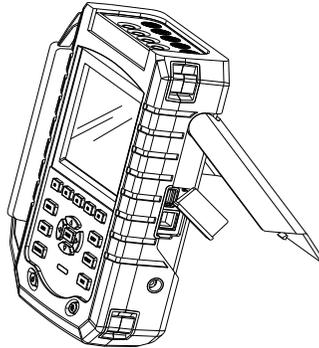
Fig. 2-1-1 Tilt stand and locations of interfaces
