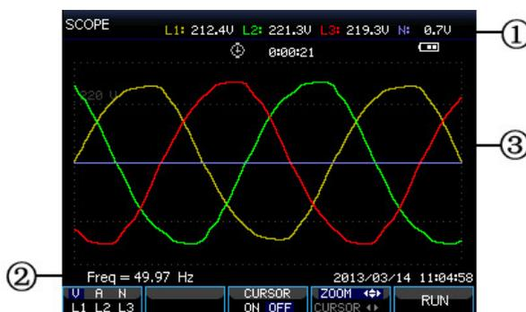
Fig. 1-5-3 Waveform screen
